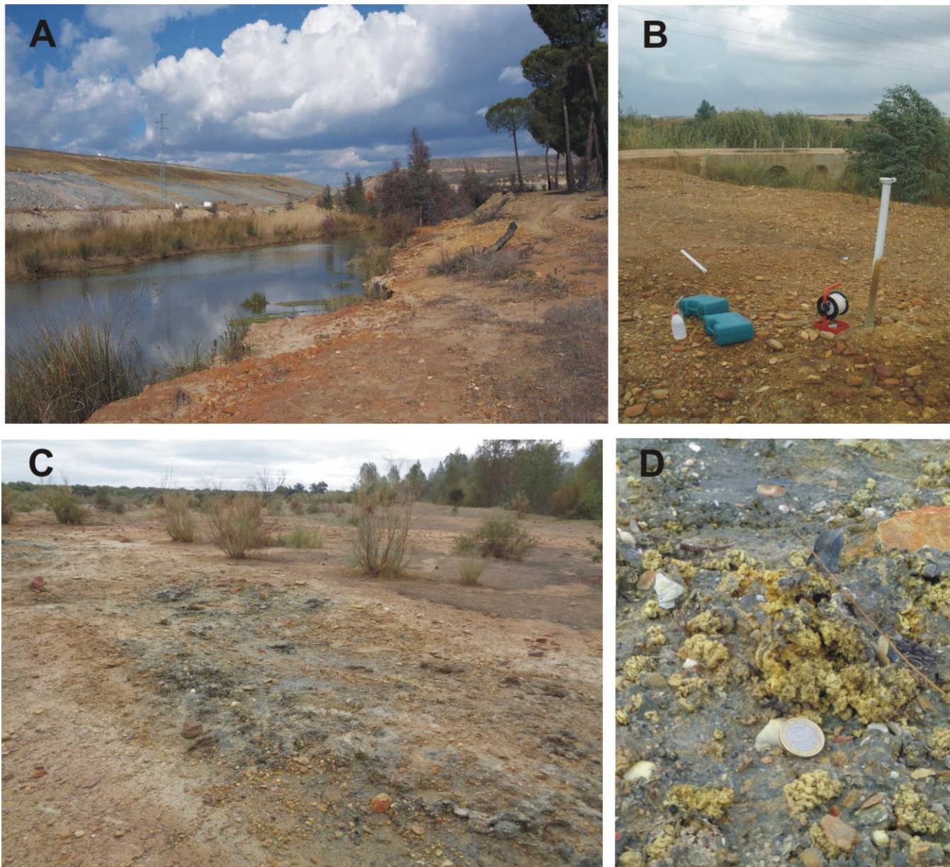
Figure 3. Photographs of the zone: A) The Agrio River at point A1, with the tailings dam wall on the left (picture looking northward), B) Sampling piezometer downstream the permeable reactive barrier (alluvial materials forming the aquifer can be observed), C) Polluted soil spot close to point A1 with grey color and scarce vegetation due to sulfide sludge remains, D) Detail of picture C showing soluble sulfate salts formed from sulfide oxidation.
