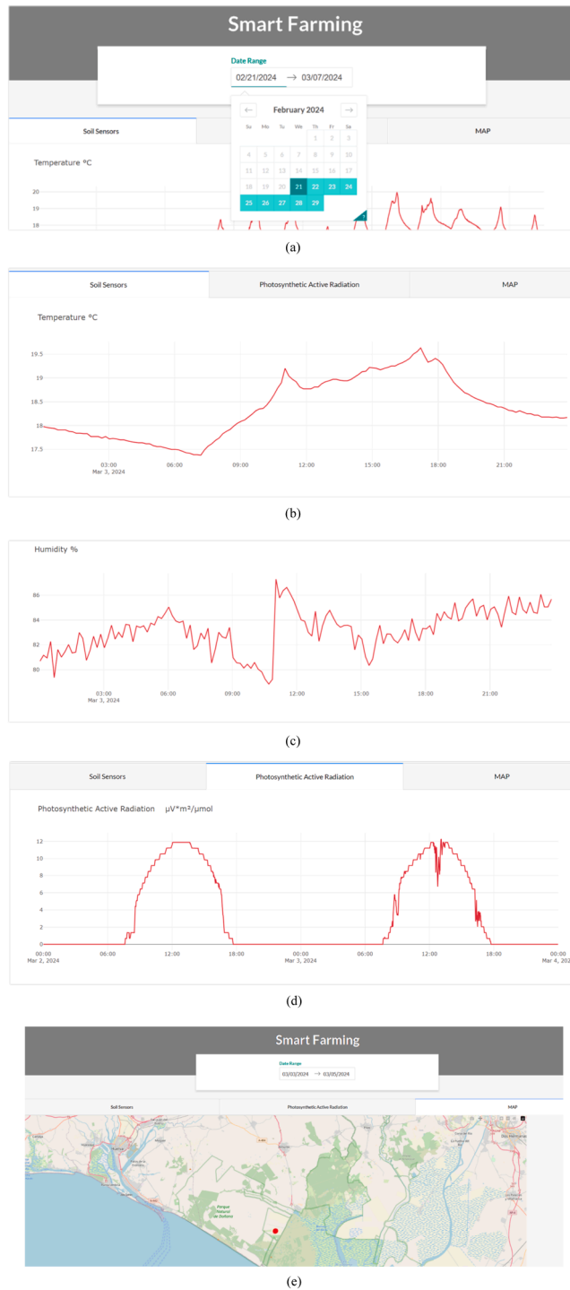
Fig. 9. (a) GUI of the irrigation system, (b) and (c) temperature and soil moisture collected data of different wireless sensor nodes, (d) Measured data of PAR sensor over two days gathered by LoRaWAN gateway node, (e) Geographic location of devices in the southwestern Spain close to the Doñana National Park and Atlantic Ocean in a strawberry plantation.
