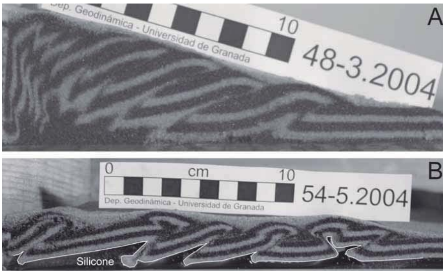
Fig. 5.- Cross-sections cut parallel to the tectonic transport direction at the end of the experiment of the models with frictional (A) and viscous substrate (B). Locations in Fig. 2D and Fig. 3B, respectively.
