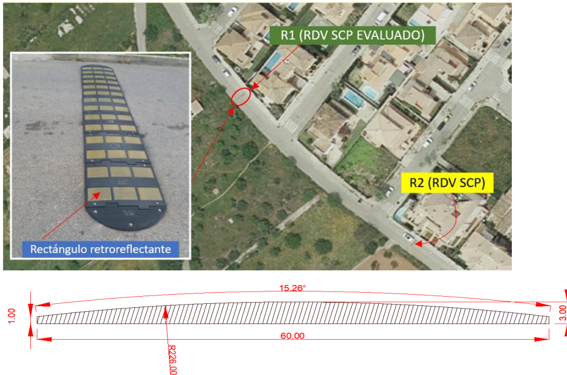
Fig. D. Top image: track section with evaluated RDV SCP. Source: image obtained from IDEIB (Spatial Data Infrastructure of the Balearic Islands) and edited by the authors. Bottom image: longitudinal section drawing of the RDV SCP.
