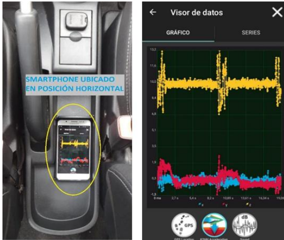
Fig. B. Location of the smartphone in the vehicle and acceleration graph in the X, Y, Z axes vs. time.
