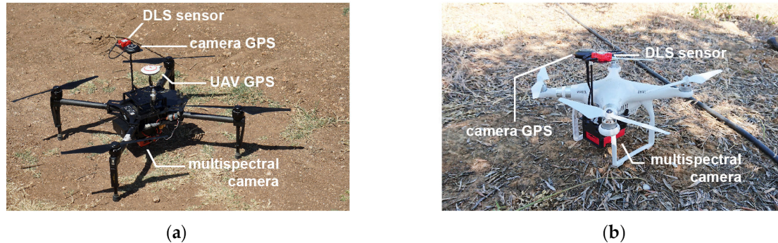
Figure 4. Aerial image acquisition equipment: (a) DJI Matrice 100-based configuration; (b) DJI Phantom 3 Advance-based configuration.
