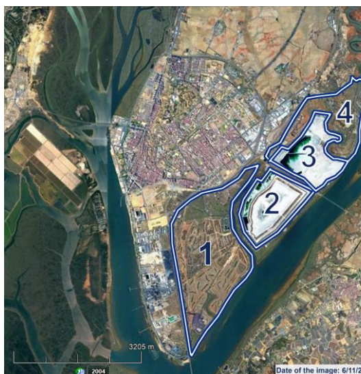
Fig. 10. Zones of the phosphogypsum deposit in Huelva. Zones 1 and 4: restored areas. Zone 2: pyramidal stack. Zone 3: PG evaporation pond.
