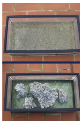
Fig. 13. Picture of the tank experiment with phosphogypsum (up), and layered salts (down).
