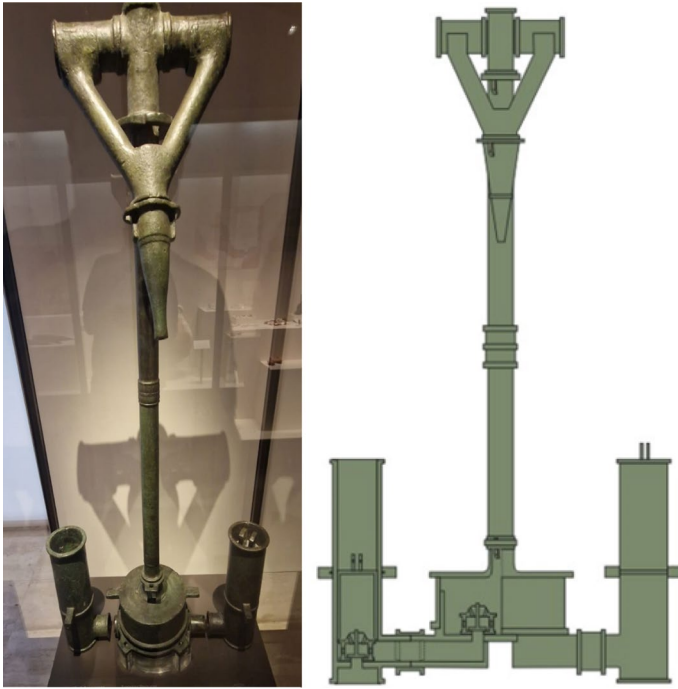
Fig. 10 Sotiel Coronada's pump, Calañas a Archaeological National Museum, (Madrid). b Draw of a Ctesibius pump (Delgado-Domínguez & Pérez-Macías, 2013)
