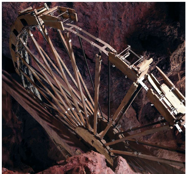
Fig. 7 Reconstruction of Hispanic type Water Wheel. Rio Tinto Mining Museum
