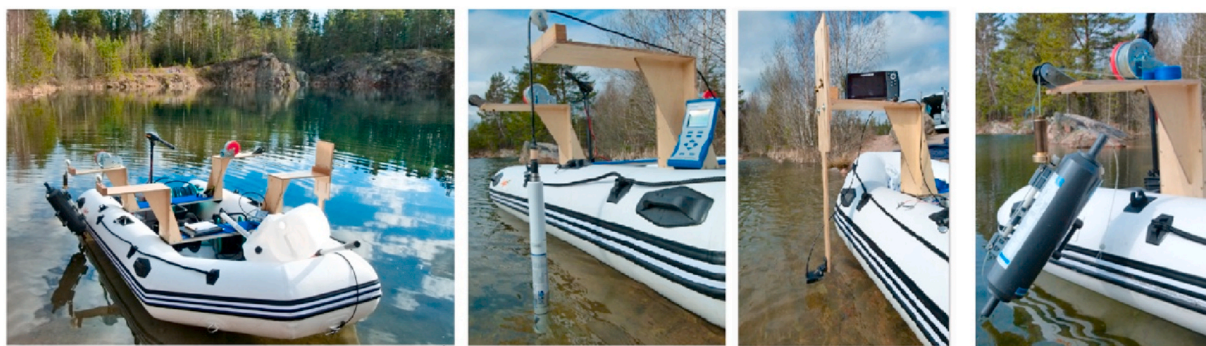
Fig. 2. Different probes and sampling systems used during this project. From left to right: the fully-equipped boat, Hydrolab M5 multiparametric water probe, Helix 551 echo sounder and Niskin bottle.
